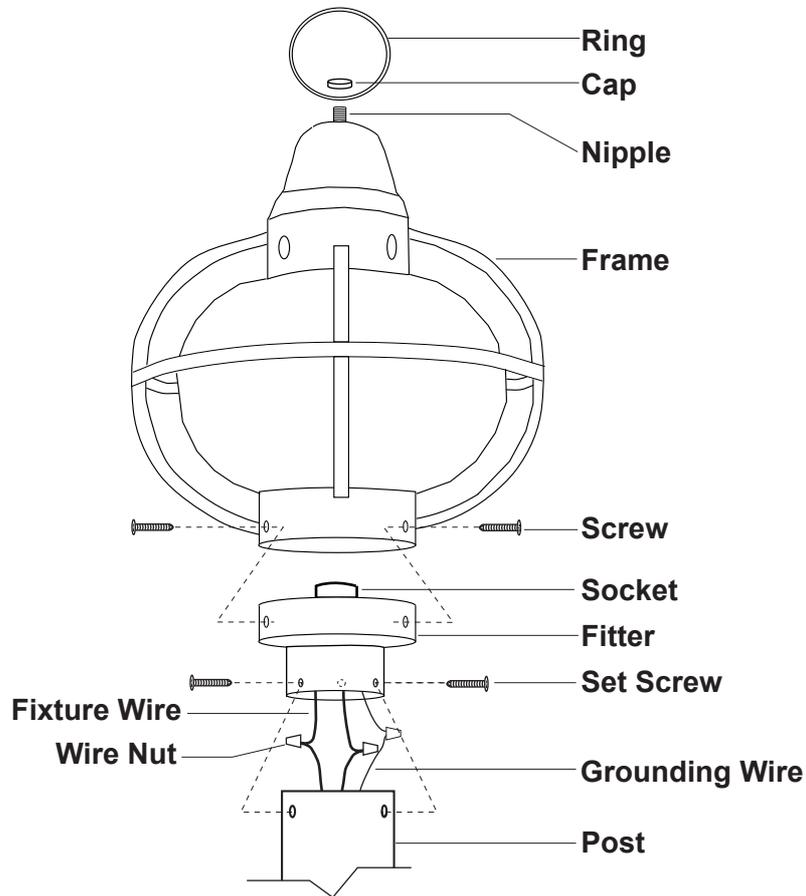
1. Unscrew the screws to remove the frame away from the fitter.
